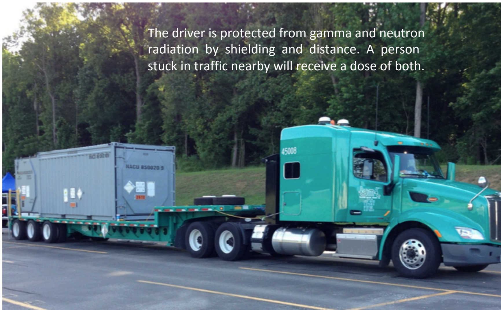
Transport Truck with ISO Container in which the NAC-LWT Cask is Carried
