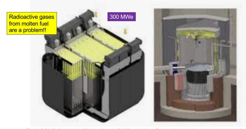
Each SOLID fuel rod is filled with a LIQUID solution of plutonium and transuranics in molten salt. The PRIMARY COOLANT is molten salt that carries heat to the SECONDARY COOLANT (water).
