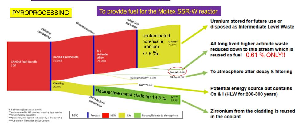
SSR Fuel = plutonium + other transuranics = 0.61 percent of the total mass of used CANDU fuel. This small fraction is used to fuel the SSR-W reactor. The other 99.39 percent is leftover waste.
