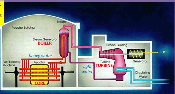
Uranium atoms are split in the CORE to heat water.
