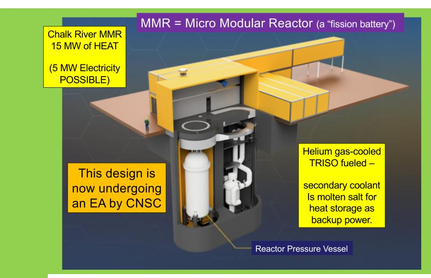
Ultrasafe MMR = Micro Modular Reactor – 15 MWth – Helium-cooled – Molten Salt storage
