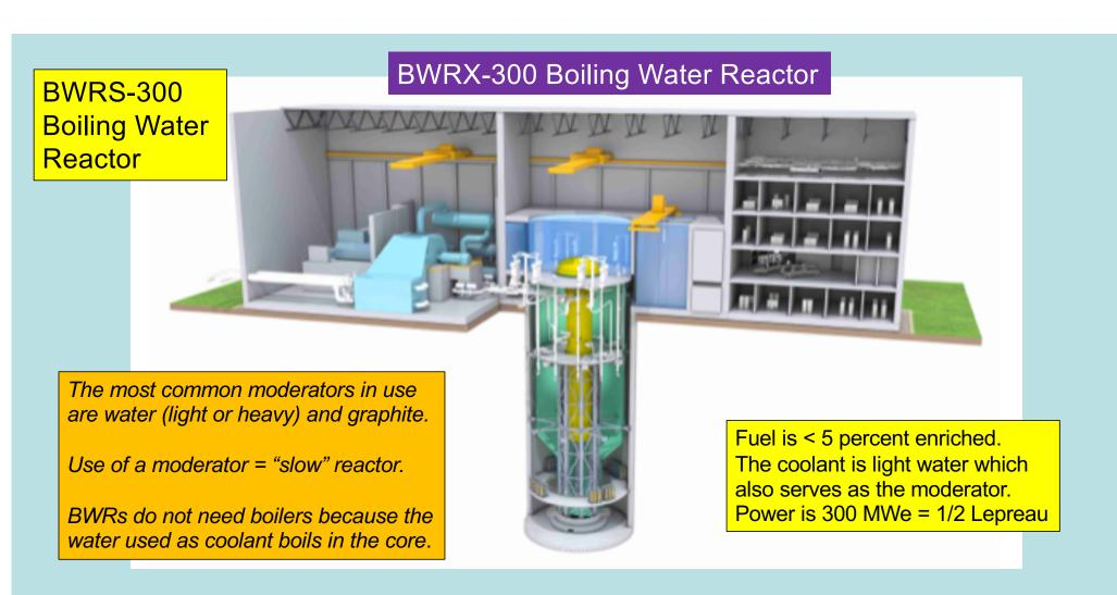
BWRX-300 = scaled down boiling water reactor – GE- Hitachi
