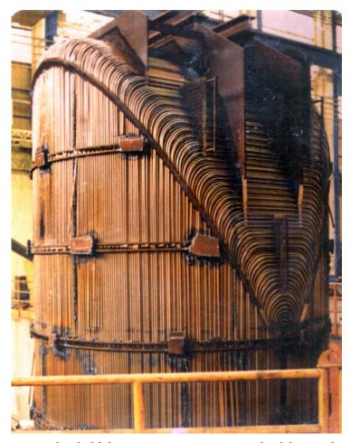
A nuclear steam generator (shown on the left) is an enormous vessel with steel walls -- a nuclear "boiler". But the water from the core of the reactor (called the "primary coolant") is not allowed to boil; instead, the primary coolant runs through thousands of small tubes that act as heating elements to boil other water called "secondary coolant". The steam from the secondary coolant is used to spin a turbine and generate electricity.
