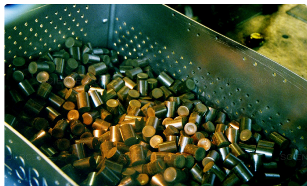
Figure 3. Sintered uranium dioxide fuel pellets
