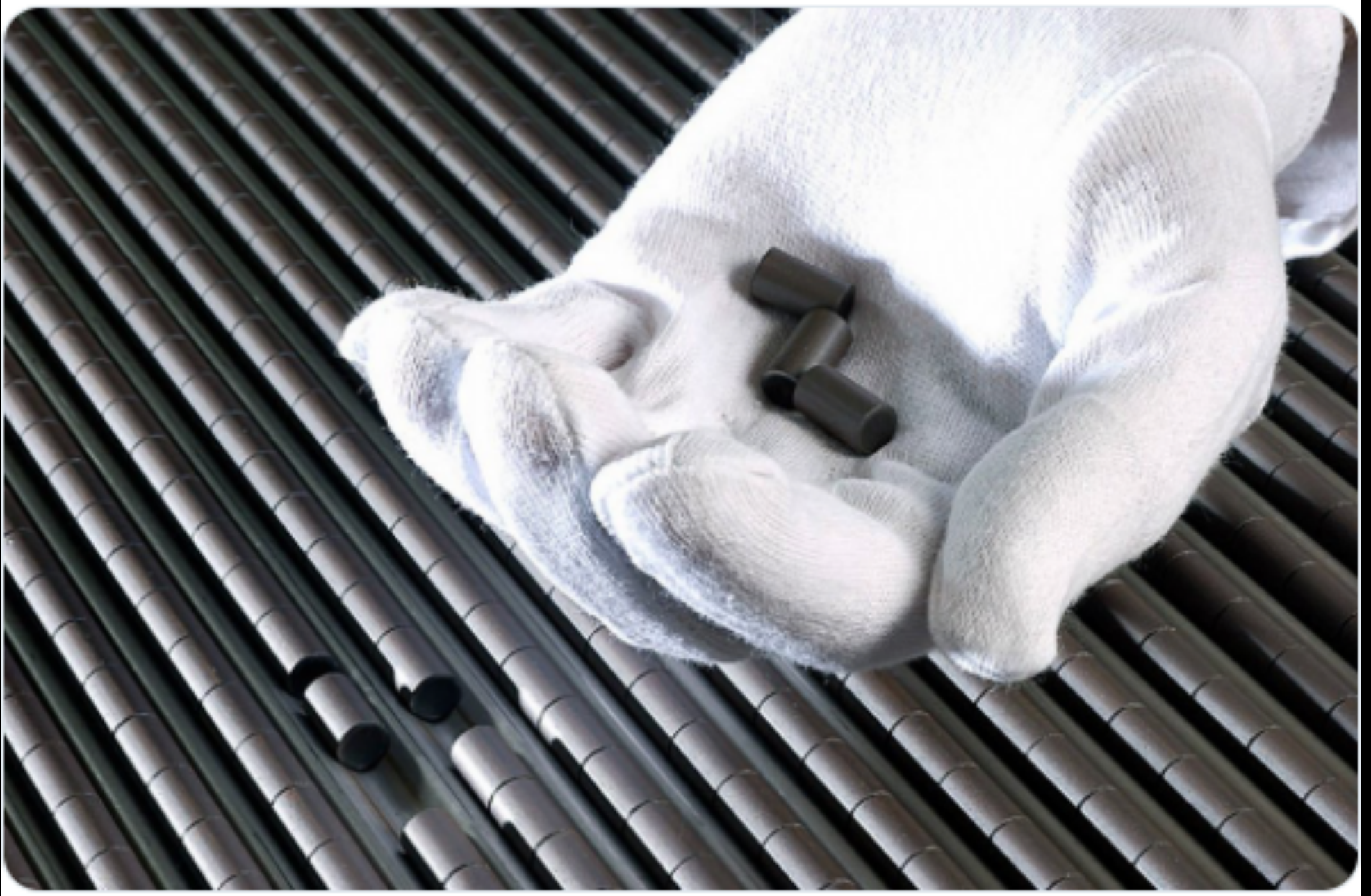
Ceramic nuclear fuel pellets are made from uranium dioxide powder
