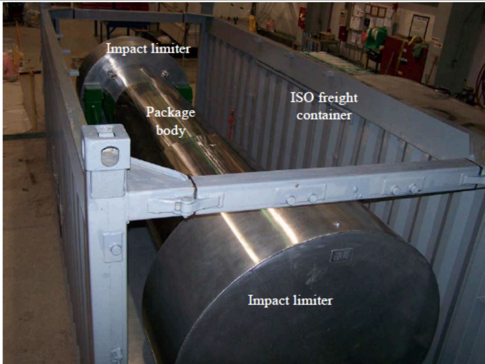
NAC-LWT cask with impact limiters, inside a truck's shipping container. The impact limiters are designed to absorb the shock of an impact.
