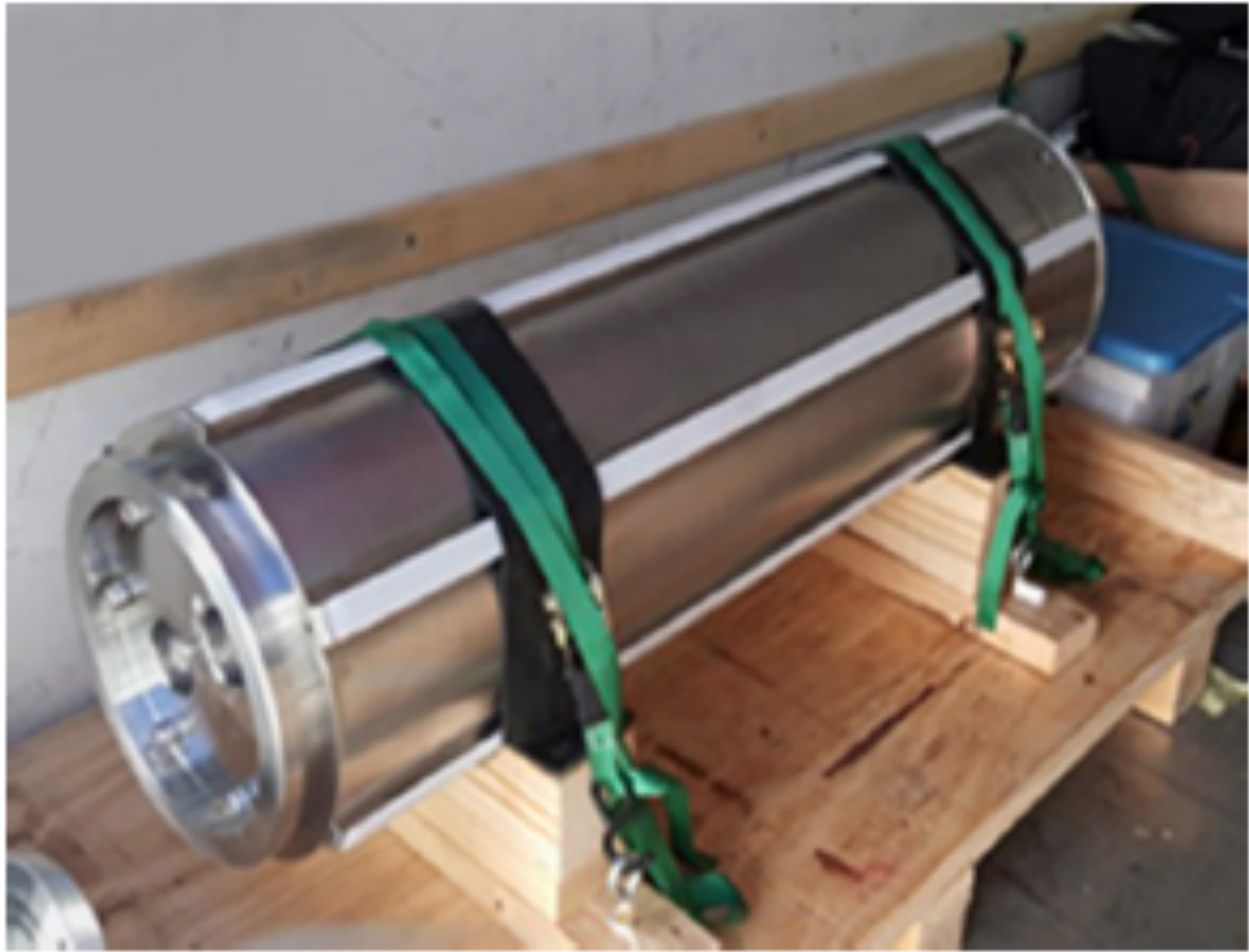
The radioactive liquid is carried in 4 inner containers placed inside the inner cavity.
