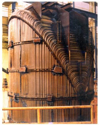
A nuclear steam generator is an enormous vessel with steel walls (this is a US model, not a CANDU). It is a nuclear "boiler".
